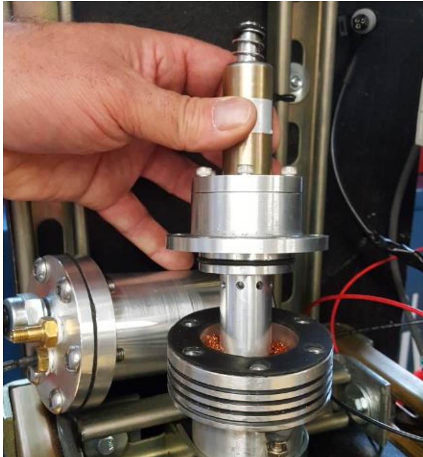
Figure 19 Inner-Grander Cylinder Interface with Flange screws removed
