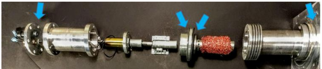
Figure 18 "Exploded View" of Stirling cooler with arrows pointing at gaskets
