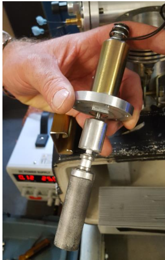
Figure 17 Solenoid-Piston-Displacer Assembly with a visual of the disc magnets
