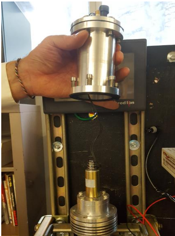
Figure 23 Disconnected Motor Housing Assembly
